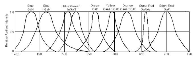
$\label{eq:wavelength} Wavelength \; \lambda \; (nm) \\ \textbf{Relative Intensity vs. Wavelength}$
