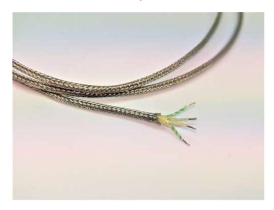
Glassfibre insulated flat pair construction, conductors laid flat, Glassfibre insulated with Glassfibre jacket, silicone varnished throughout + stainless steel overbraid for added protection and mechanical strength. Good temperature resistance but not suitable where fluids are present.
