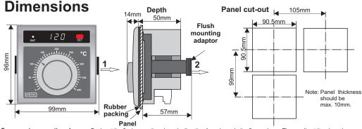
For removing mounting clamps: Push out the flush-mounting clamp in direction 1 as shown in the figure above. Then, pull out the clamp in direction 2. If there is no 60mm free space at back side of the device, it would be difficult to remove it from
