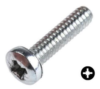
Pan Head machine screws, similarly to Oval Head machine screws have rounded sides, however the difference being that Pan Head machine screws have a flat top rather than a rounded one. The cross recess drive, also known as Posidriv, is becoming a popular method with this type of fastener due to ease of assembly with reduced driver slippage (Cam Out) which reduces the effect of surface damage. Machine screws can be used in pre-tapped holes or used with conforming nuts and washers in through-holes.
