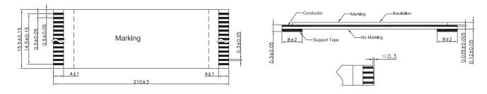
Dimensions : Millimetres Tolerances: ±0.3mm
