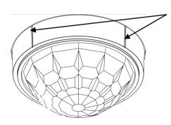
The sensor head has 4 alignment marks. These correspond to the 4 outer passive infrared sensors under the lens. Use these marks to align with aisles and corridors to ensure the best detection characteristics. See example overleaf.
