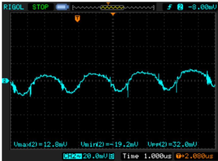
Figure 3. Output ripple at 8A load.
