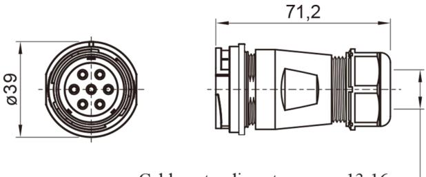
Cable outer diameter range: 13-16mm
