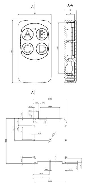
All dimensions are given within +/-0,5mm tolerance
