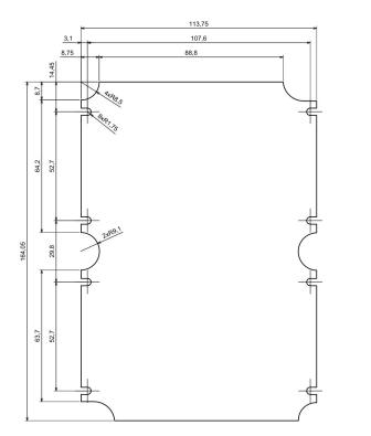
All dimensions are given within +/-0,5mm tolerance
