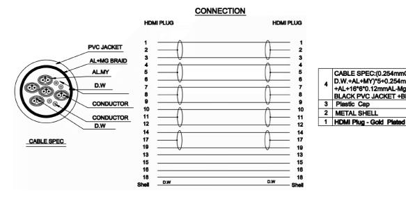
CABLE SPEC:(0.254mmCu\*1Pair+0.254mmCu D.W.+AL+MY)\*5+0.254mmCu\*4C+0.254mmCu D.W. +AL+16\*6\*0.12mmAL-Mg Braiding)\*1C O.D:6.3mm BLACK PVC JACKET +BLACK NYLON BRAIDING
