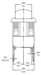
Dimensions : Inches/Millimetres Tolerances ±0.012"/0.3mm
