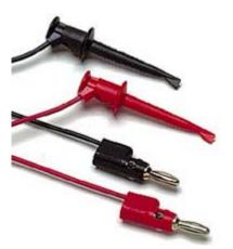
1 pair (red, black) of test leads with multi-stacking 4 mm banana plugs and mini-hooks Mini-hooks attach to component leads up to 1.5 mm diameter 90 cm long PVC insulated leads 30 V rms or 60 V DC, 5 A One year warranty
