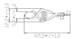
MATERIALS: STEEL, NICKEL PLATED UNIT:MM
