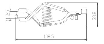
MATERIALS: STEEL, NICKEL PLATED UNIT:MM
