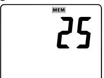
② Press "READ" key to enter the manual memory data mode. The LCD display will show " READ " and a memory location number.
