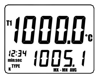
T1 present reading + T1 Maximum reading plus elapsed time + T1 Minimum reading plus elapsed time + T1 Averaging reading plus averaging time.
