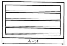
Louvres are manufactured in one piece units up to 1800mm square.
