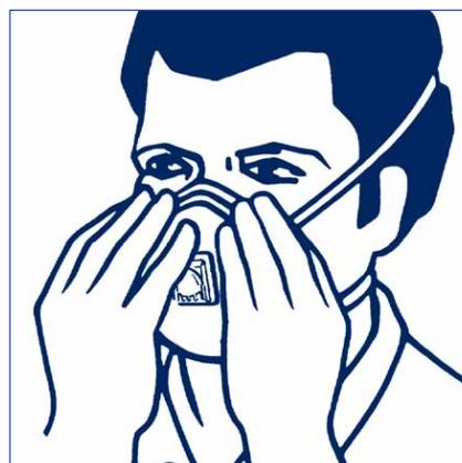
5. The seal of the respirator on the face should be fit-checked prior to wearing in the work area.
