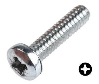
Pan Head machine screws, similarly to Oval Head machine screws have rounded sides, however the difference being that Pan Head machine screws have a flat top rather than a rounded one. The cross recess drive, also known as Posidriv, is becoming a popular method with this type of fastener due to ease of assembly with reduced driver slippage (Cam Out) which reduces the effect of surface damage. Machine screws can be used in pre-tapped holes or used with conforming nuts and washers in through-holes.
