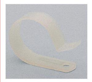
Material: UL approved Nylon 66, 94V-2 KSS CABLE CLAMPS are designed to hold cable, tubes, and components in domestic appliance, electronics and electric apparatus generally. Interior edges are radiused to protect cable insulation. To apply, just clamp down on loosen cables and screw it to chassis. Black colour available
