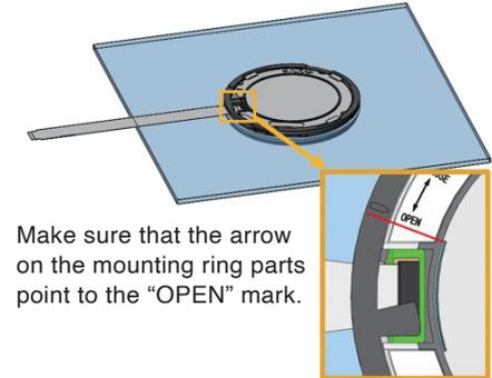
Make sure that the arrow on the mounting ring parts point to the "OPEN" mark.
