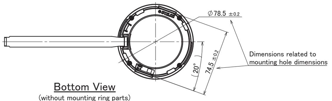
Tolerance without indication is  $\pm 1.0\text{mm}$
