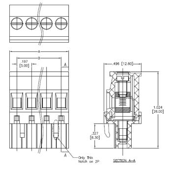
Positions: 02 thru 24 A = .197 [5.00] x No. of Positions B = .197 [5.00] x No. of Spaces
