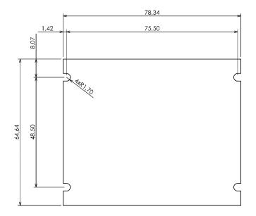
All dimensions are given within +/-0,5mm tolerance
