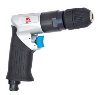
RS Pro Air Drill, 10 mm keyless chuck air drill with a magnesium body. Lightweight feel and a high performance motor maximise output speed. Ergonomic grip design for better manoeuvrability, while the durable motor designed with high balance for precision work without vibration. Speed control trigger for precision work and a thumb lever to switch drive direction with one finger.
