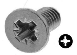
Countersunk, also known as Flat Head Machine Screws, are designed for ease of assembly and these machine screws with their cross recess drives are a popular driving method with this type of fastener as they allow the head to sink into the material. Machine screws can be used in pre-tapped holes or used with conforming nuts and washers in through holes.
