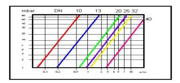
Schedule 2: Pressure loss for type of end connection based in internal diameter (DN)
