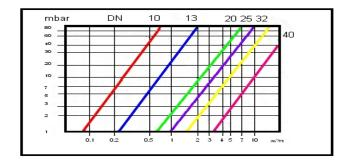
Therefore pressure drop (mbar) can be calculated for any given hose assembly adding P1 and P2.
