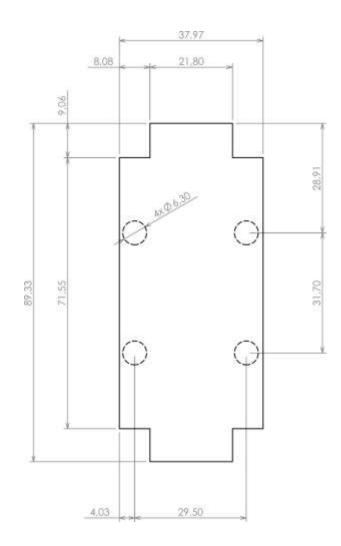
Dashed line shows outline of the mounting boss under PCB board Recommended mounting holes diameter ø3,5mm All dimensions are given within +/-0,5mm tolerance
