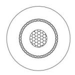
Cable Marking: RS PRO 1 Core×0.5mm<sup>2</sup>
