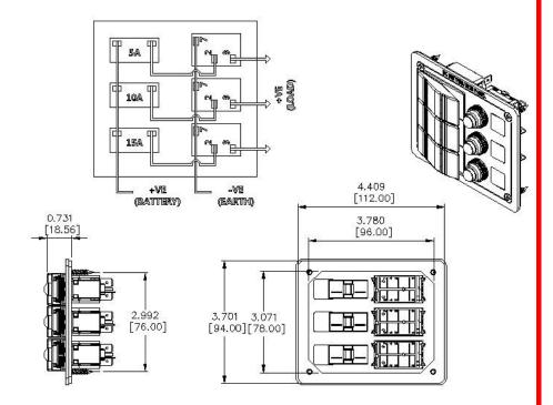
Rocker Switch x 3 (SPST / ON-OFF) 5A Breakers  $\times$  1
