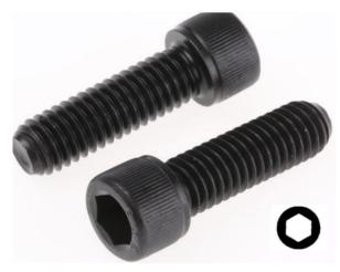
Socket Caps have a small cylindrical head with tall, vertical sides giving them space saving advantages as well as greater tensile strength. They also require less side room for wrenches. These socket screws are used in many applications including the manufacture and repair of vehicles, machine tooling, tools and dies, machine production and repair and general engineering applications. Most importantly, socket cap head screws provide safety, reliability and cost efficiency.
