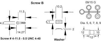
Dimensions : Millimetres Tolerance: ±0.5mm
