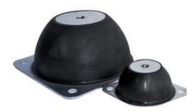
High Deflection Motor Mounts are ideal for applications that require high deflection under low loads while operating under low frequencies. Flexible in all directions, this mount is also an ideal product for shock applications by deflecting and returning to its original shape.
