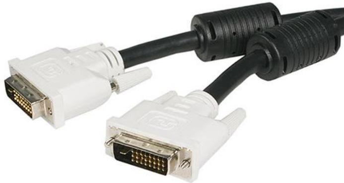
The DVIDDMM5M 5m DVI-D Dual Link cable features 2 male DVI (25-pin) connectors and offers 5 meters in cable length, making it perfect for longer connections between your desktop or laptop computer and a DVI-D monitor or projector.
