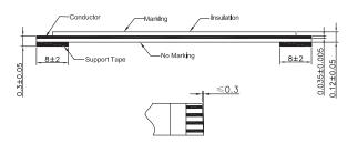
Dimensions: Millimetres Tolerances: ±0.3mm
