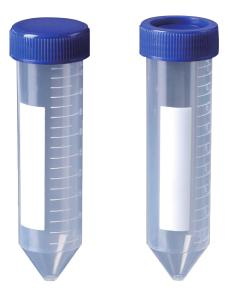
Graduation Range: 5-47.5ml Graduation Interval: 2.5ml Autoclavable: at 121°C Freezable: -45°C Maximum RCF: 9,500xg Dimensions tube: 29D x 115L mm Performance: Dnase/Rnase-free Non-pyrogenic<0.25 EU/ml FDA Registered
