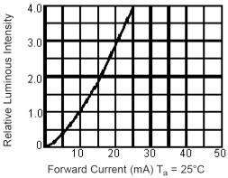
Luminous Intensity vs. Forward Current
