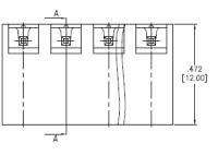
Positions: 02 thru 24 A = .200 [5.08] x No. of Positions B = .200 [5.08] x No. of Spaces
