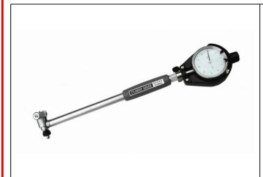
The Dial Bore Gauge provides a two point measuring system for comparative measurement of component hole sizes. It will also detect ovality and taper in bores These instruments are fitted with spring loaded centralising mechanisms which ensure the measurement is taken across the true diameter of the component. All instruments are supplied in cases complete with probes and extensions as listed
