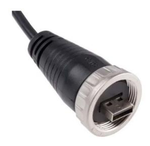
The RS PRO series of waterproof metal USB-A connectors are a range of ruggedised IP67/IP68 connectors designed to be used outdoors or in harsher industrial environments. Designed to fit panel cut outs of 25.5mm the metal USB-A series also comes with rear potting on the panel mount connectors. This ensures your panel is still sealed to an IP67/IP68 rating even when the connector is unmated, and the sealing cap is not connected. The threaded mating allows for a secure connection.
