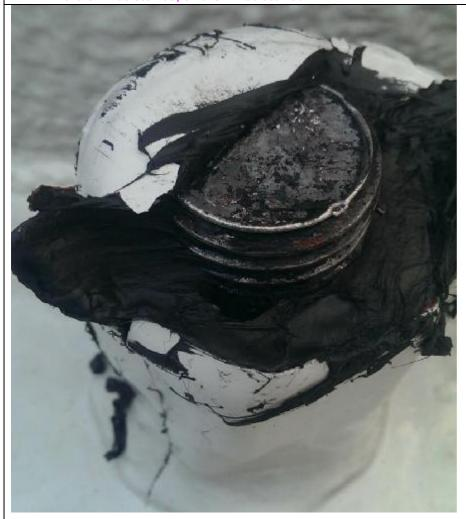
One year no any corrosion (top of Bolt surface is still showing Metallic Luster, which same as the original status). Tip: Enlarge the PDF file to see the photo in details
