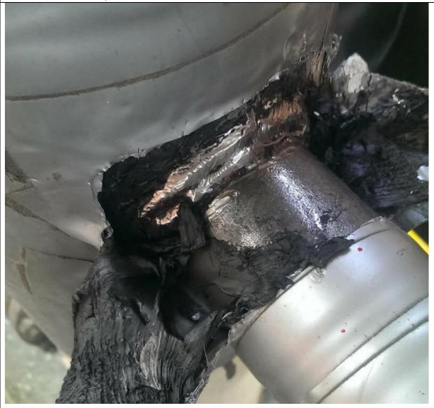
One year no any corrosion (both Weld End and Pipe's surface is still showing Metallic Luster, which same as the original status). Remark: the Brown color was the primer of paint which is the Surface Preparation of pipe did not good enough) Tip: Enlarge the PDF file to see the photo in details.
