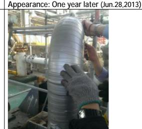
1 year Demo Test Result: June 28, 2013\_Peel-off to check (= No any corrosion) = EXCELLENT Water & Air Immersion Resistance, and UV Resistance.
