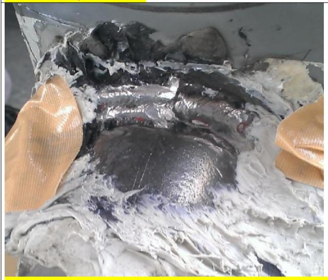
Two year no any corrosion (both Weld End and Pipe's surface is still showing Metallic Luster, which same as the original status).
