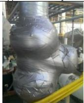
1 year Demo Test Result: June 28, 2013\_Peel-off to check (= No any corrosion) = EXCELLENT Water & Air Immersion Resistance, and UV Resistance.
