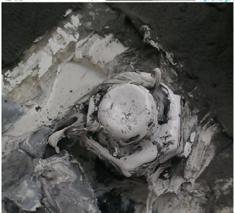
Remark: This object's surface didn't made any of Surface Preparation before demo test (= had Paint), In normal condition, the Paint cannot Anti-Corrosion within half or one year in the coastal region (= serious corrosion environment). This demo test is focusing the IMMERSION RESISTANCE (Water Tight & Air Tight) for the reinforcement to Nut group and for Anti-Corrosion. (and required easy to be apply)
