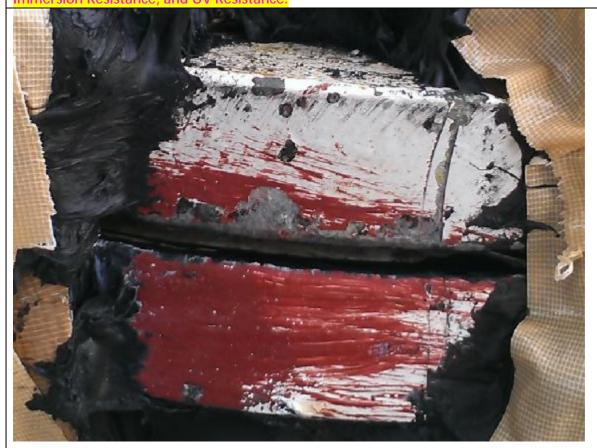
One year no any corrosion (the Flange's surface and Gap are still showing Metallic Luster, which same as Remark: the Brown color was the primer of paint which is the Surface Preparation of pipe the original status). did not good enough) Tip: Enlarge the PDF file to see the photo in details.
