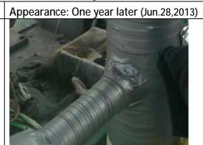
1 year Demo Test Result: June 28, 2013\_Peel-off to check (= No any corrosion) = EXCELLENT Water & Air Immersion Resistance, and UV Resistance.
