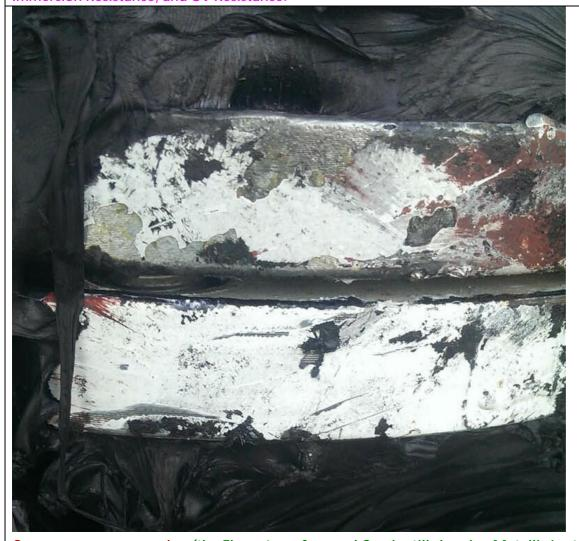
One year no any corrosion (the Flange's surface and Gap is still showing Metallic Luster, which same as the original status). Remark: the Brown color was the primer of paint which is the Surface Preparation of pipe did not good enough) Tip: Enlarge the PDF file to see the photo in details.
