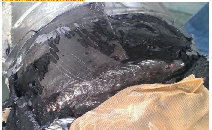
Two year no any corrosion (both Weld End and Pipe's surface is still showing Metallic Luster, which same as the original status).
