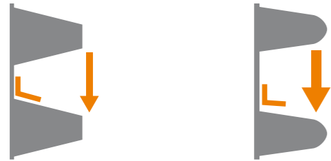
Steeper thread angle, standard geometry
