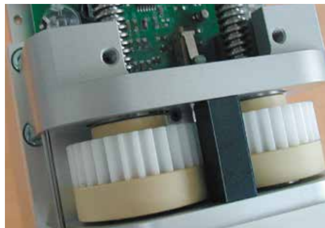
This mixing station uses two drylin® trapezoidal lead screw nuts made from iglidur® high-performance polymers for the optimal mixing ratio of a two-component silicone mass.
