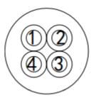
Cable Marking: RS PRO 4 Core×0.25mm<sup>2</sup> Unscreened Industrial Cable 250V
