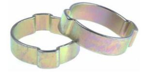
The RS Pro range of double ear O clips also known as lemon clips, 2 ear clips or double ear clips come in a range of sizes starting with a 5mm minimum diameter to 27mm maximum diameter, starting from a 6mm band width to 10mm.
