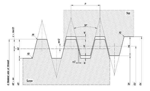
$$\begin{split} &H_1 = 0.5 \; P \\ &h_3 = H_4 = H_1 + a_c = 0.5 \; P + ac \\ &z = 0.25 \; P = H_1/2 \\ &d_3 = d - 2 \; h_3 \\ &d_2 = D_2 = d - 2 \; z = d - 0.5 \; P \\ &D_2 = d + 2 \; a_c \\ &a_c = bottom \; play \\ &es = top \; deviation \; for \; screw \\ &s = 0.26795 \; es \\ &R_1 \; max. = 0.5 \; a_c \\ &R_2 \; max. = a_c \end{split}$$
