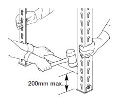
To locate beams: Clip lugs at the ends of the beam into the 'P' slots in the upright. Press down, then tap into place ensuring lugs are fully located to the base of the slots.
