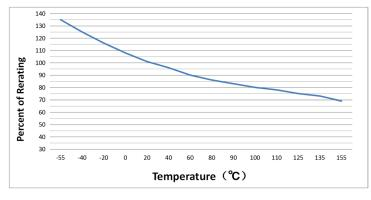
Normal ambient temperature:  $23 \pm 3^{\circ}$ COperating temperature:  $-55^{\circ}$ C ~ +150°C, with proper correction factor applied
