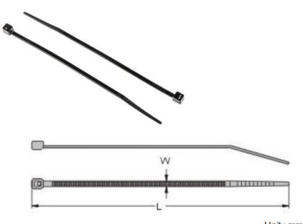
Unit: mm Length Min Loop Tensile Max. L Width W Bundle Strength Item No. packing Dia. mm inch lbs kgs 4" 2.5 5 1/2" 3.2 7 1/2" 4.8 8" 4.6 9 7/16" 7.6 11 7/8" 4.8 100PC/BG 11 7/8" 7.6 15" 7.6 15 3/16" 4.8 17 3/4" 4.8 17 3/4" 24" 29 1/2" 7.5
