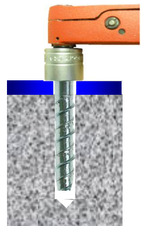
Tighten with torque wrench to recommended torque
