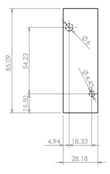
Dashed line shows outline of the mounting boss under PCB board Recommended mounting holes diameter ø3,5mm
