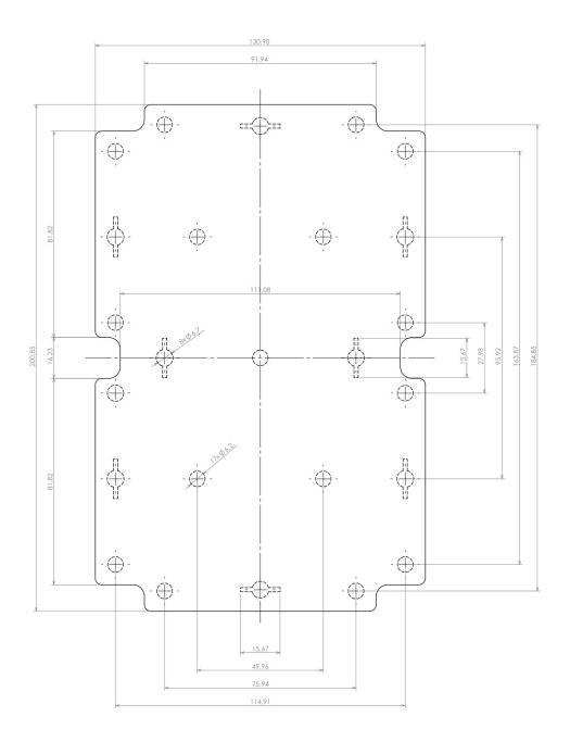
Dashed line shows outline of the mounting boss under PCB board Recommended mounting holes diameter ø4mm All dimensions are given within +/-0,5mm tolerance
