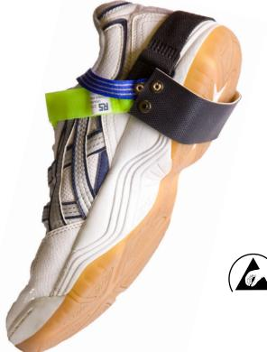
Unless otherwise noted, tolerance ±10% Specifications and procedures subject to change without notice. The heel grounder is constructed using a 36mm wide strip of two-layered rubber sheet with an insulative white and a conductive black layer attached to a 25mm wide elasticated back forming a heel cup. The heelgrounder has a 1 megohm resistor joined in series with the conductive tab. It is assembled with a separate hook and loop tape for adjustment.
